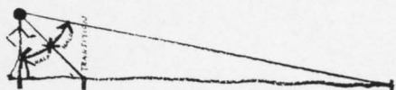
EQUAL DIVISION OF SIGHT ANGLE BRINGS POINT OF TRANSITION CLOSE TO OBSERVER
