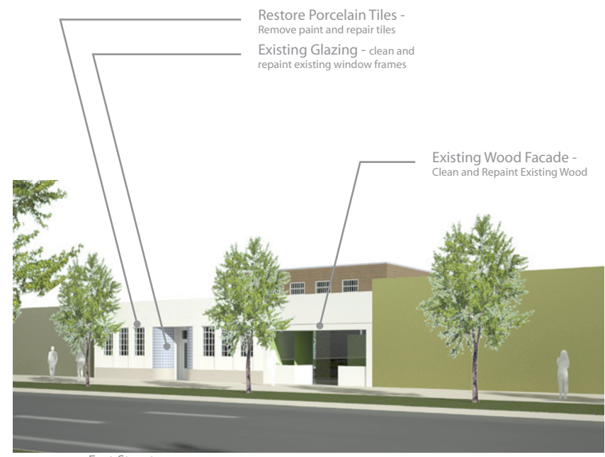
Fort Street Restored Mellus Facade
