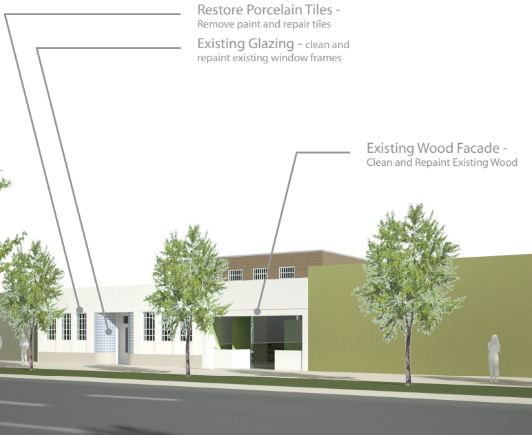
Fort Street Restored Mellus Facade
