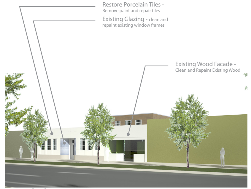
Fort Street Restored Mellus Facade
